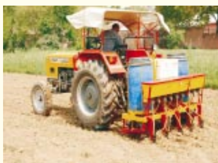
A tractor drawn gravity feed aqua-ferti-seed drill
