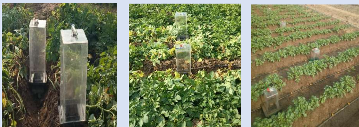
Fig 5: Sampling of nitrous oxide emission with drip fertigation in potato crop
