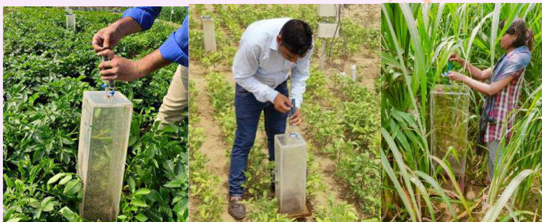
Fig 3. Sampling of GHG emission using close chamber technique in different crops
