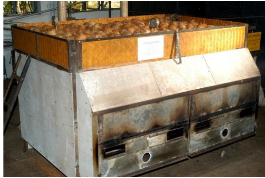
Fig. 2: Shell Fired Copra Dryer
