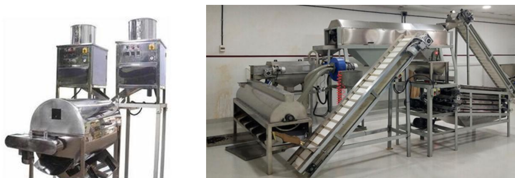
Fig. 6. Mechanized abrasion and pneumatic based peeling machine
