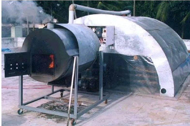
Fig. 4 : Solar cum electrical dryer with agricultural waste as third source of energy
