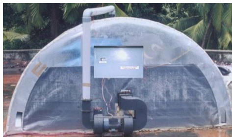
Fig. 3: Solar tunnel dryer with electricity as an alternate source of energy
