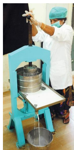
Fig. 13: Manually operated Coconut Milk Extractors
