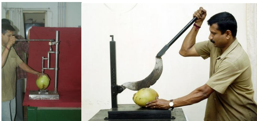
Fig. 19: Tender Coconut Handy Punch cum Splitter
