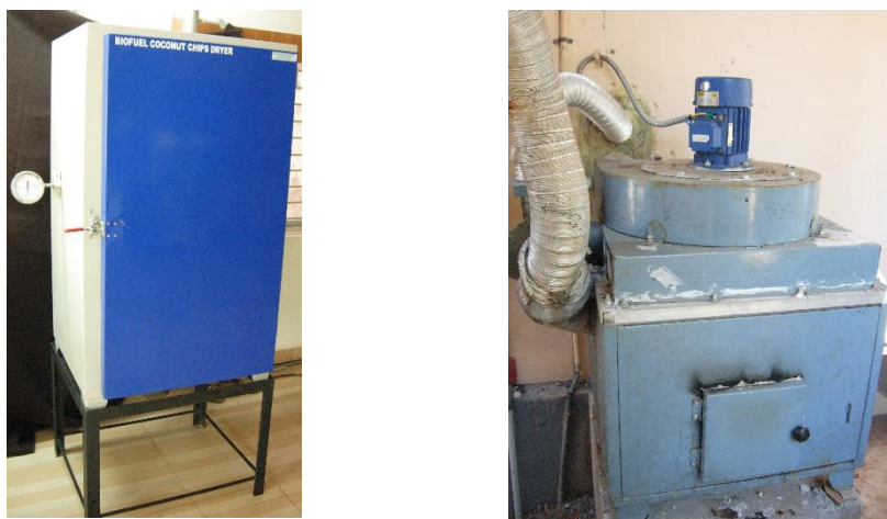
Fig. 9: Electrical and Agricultural waste fired coconut chips dryer
