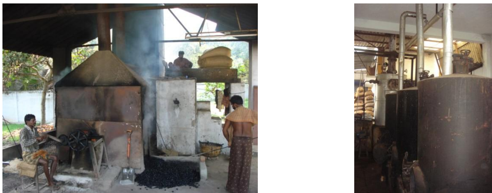
Fig 4. Drum roasting and Steam conditioning process of raw cashewnuts
