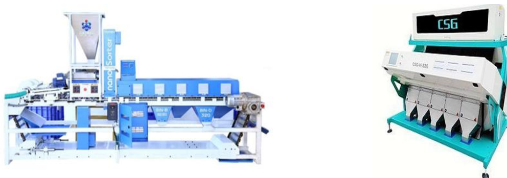
Fig 7. Size and colour-based cashew kernels graders
