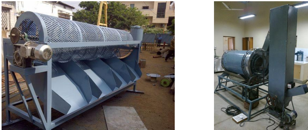
Fig 3. Calibration of raw cashewnuts
