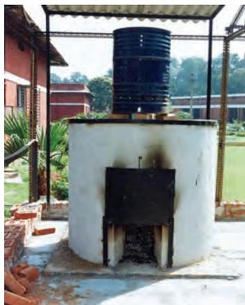
*Fig. 6. Low-cost pyrolysis kiln for preparation of biochar
