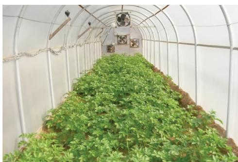
Temperature gradient tunnel (TGT)
