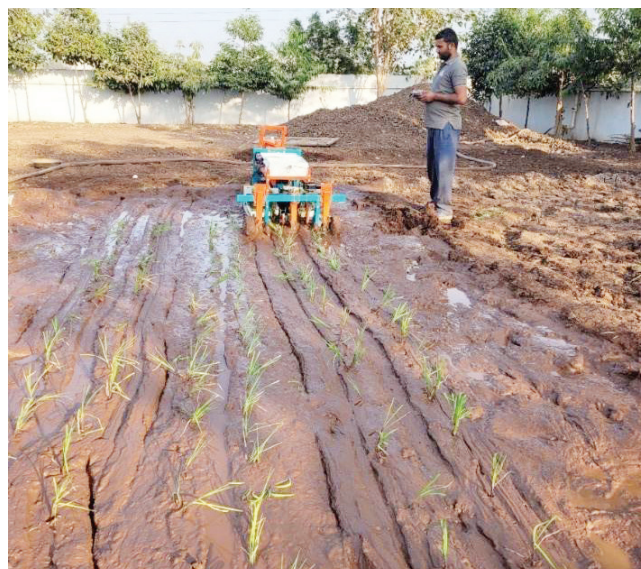
Robotic root washed type paddy transplanter
