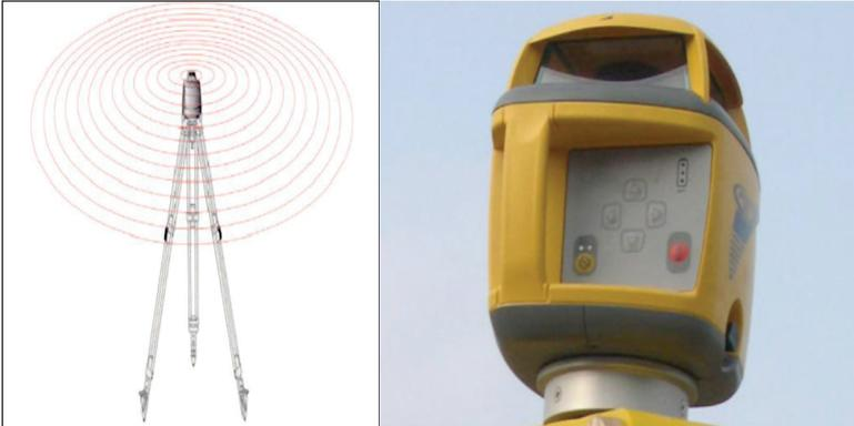
**Fig. 1.4: Laser transmitter**
