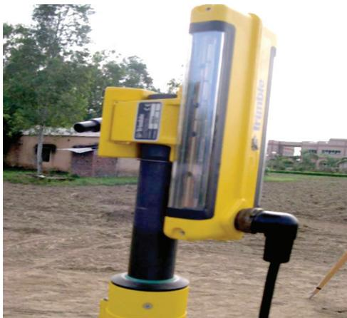
**Fig. 1.5: Laser receiver**
