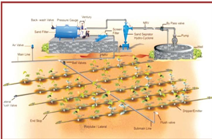
**Fig. 5.5: Drip irrigation system**
