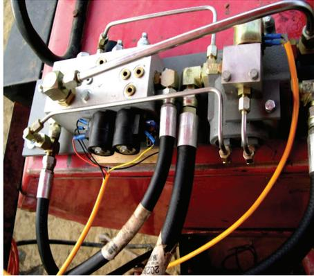
**Fig. 1.7: Hydraulic control system**
