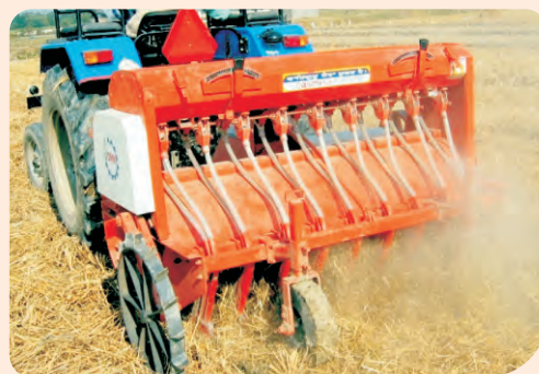
Happy seeder for sowing under zero-till residue retention situation
